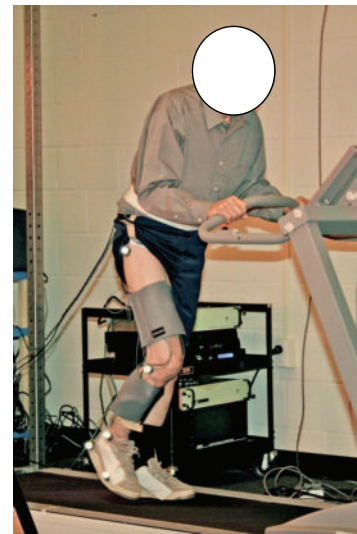
FIGURE 3: Reflective markers were placed on the hip, knee, ankle, heel, and toe (modified) to calculate the heel contact. In addition, EMG sensors were located on the right rectus femoris, tibialis anterior, lateral gastrocnemius, soleus, vastus medialis, and biceps femoris, and two workout wraps were used to stabilize the EMG sensors during faster gait speed. The subjects were instructed to hold the safety bar installed on the treadmill to avoid excessive anterior-posterior movements.
