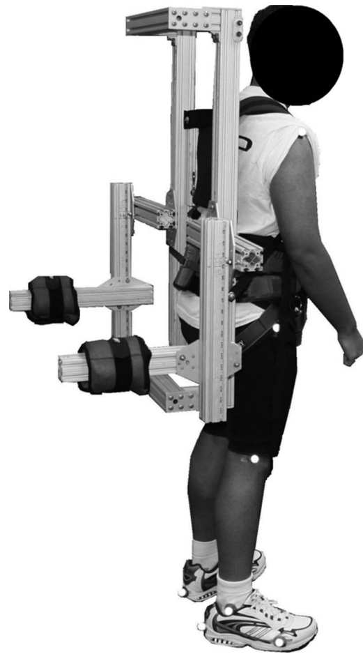
Fig. 3 Demonstration of how the PLSS rig fits on a participant. Backpack straps and a waist belt secure the rig onto the participant. Weights were applied to the back extrusions of the PLSS rig to create the aft condition here. Retroreflective markers were placed on the participant's heel, metatarsal-phalange joint, lateral malleolous, lateral epicondyle, greater trochanter, and acromion-clavicle joint.
