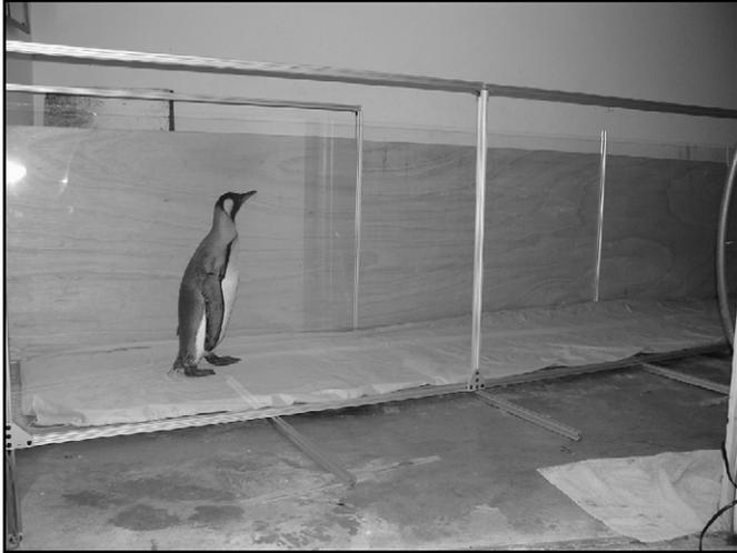
Fig. 1. The penguin walked down a custom-built walkway that had a Gaitrite pressure mat embedded in the walkway. The pressure mat registered the digital footprints for every step of the penguin's gait.
