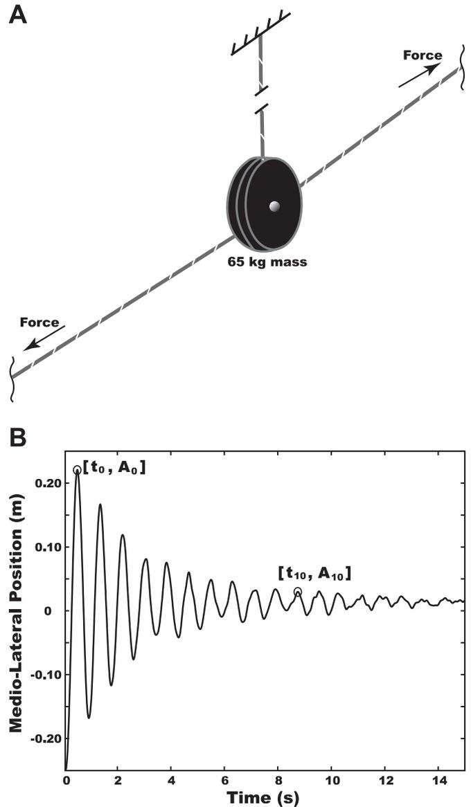
Fig. 4. Experimental set-up (A) and the mediolateral decaying oscillation of a known mass attached to the external LS system (B). Assuming a one-degree of freedom oscillation, we can compute the effective stiffness, damping ratio, and damping of the system (see APPENDIX B).
