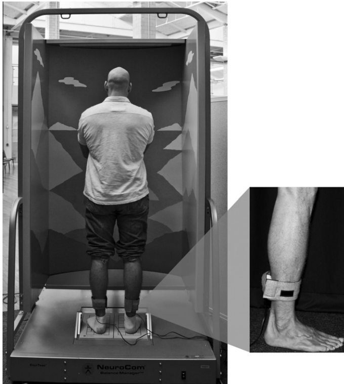
Fig. 1. Experimental setup for the current study. Force platform (NeuroCom Balance Manager) and Ia-afferent stimulation applied via local muscle tendon vibration (TechnoConcept VB 115).
